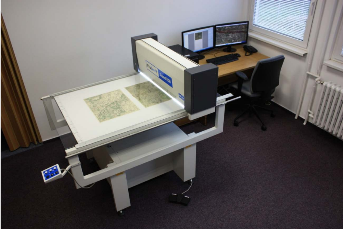
Fig. 1 The large format flat-bed scanner ScannTech 800 with 800dpi optical resolution
