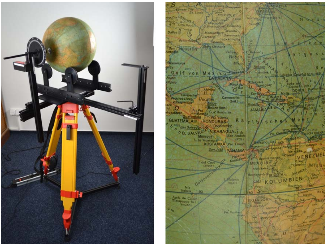
Fig. 3 New device for globe digitizing and an example of digital picture of globe
