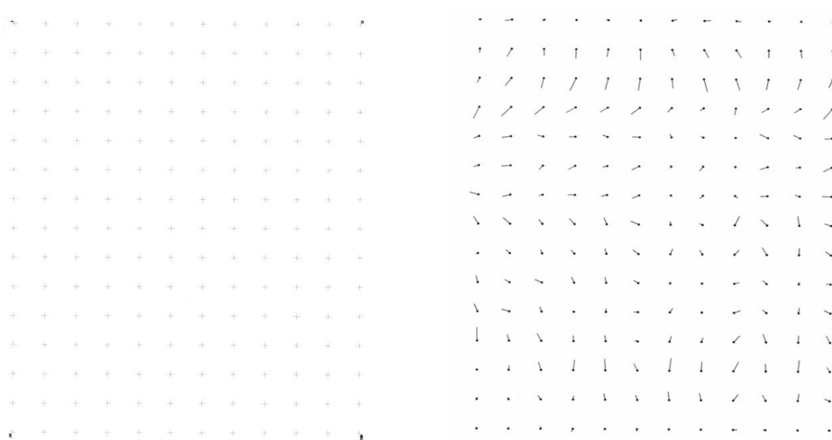
Fig. 2 Plastic used for scanner accuracy testing and the result of testing with vectors of movement
