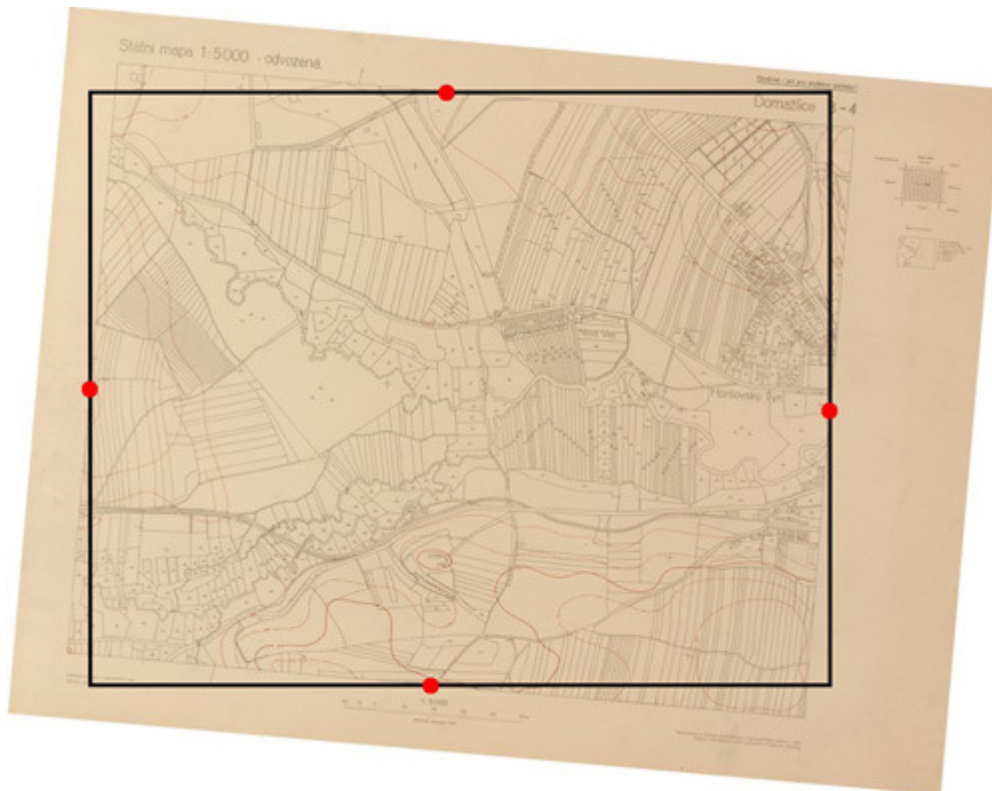
Fig. 8 - Loss of map drawing when cropping simply to map frame edges
