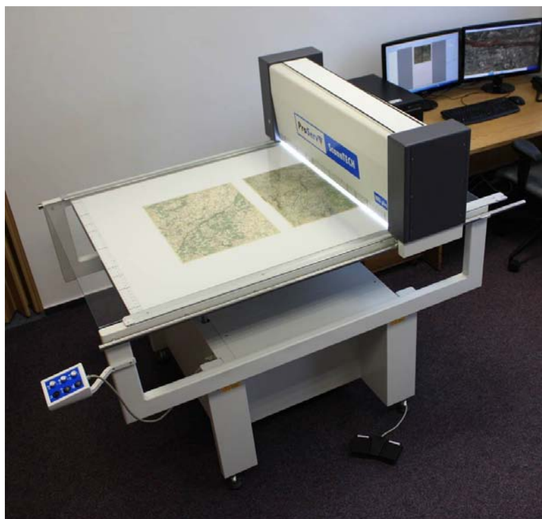
Figure 1: Large format flatbed scanner ScannTech 800i.
